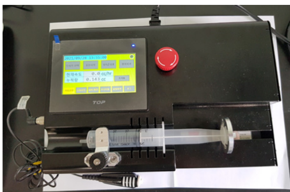
Fig. 3. Manufactured patient-controlled sedation pump that is composed of a lead screw and a stepping motor for plunging the syringe piston with a handset button.
